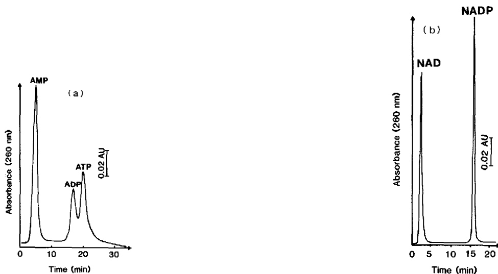
Fig. 6. Chromatography of nucleotides and coenzymes on aluminium (hydr)oxide phosphate-agarose. Column dimensions: 30 mm \times 6 mm I.D. Flow-rate: 1 ml/min. (a) Sample: 50 \mu\text{g} of each nucleotide (AMP, ADP and ATP) in a total volume of 150 \mu\text{l} . Elution: a linear gradient of potassium phosphate from 0 to 0.4 M over 30 min in 0.01 M sodium cacodylate, pH 7.0. (b) Sample: 50 \mu\text{g} of each coenzyme (NAD and NADP) in a total volume of 100 \mu\text{l} . Elution: a linear gradient of potassium phosphate from 0 to 0.4 M over 20 min in 0.01 M sodium cacodylate, pH 7.0.
